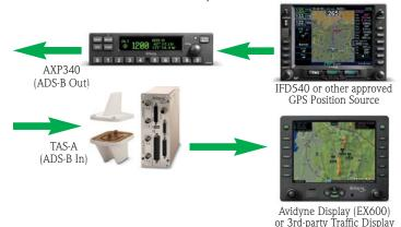
The AXP340 & TAS-A combine to provide complete 1090MHz ADS-B solution. ADS-B & TAS traffic can be displayed on a wide range of displays including Avidyne's EX600 (shown here), providing the highest level of situational awareness and safety.
