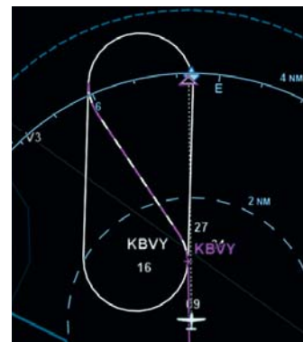
The segmented magenta line makes it very easy to see the next leg in the flight plan.
