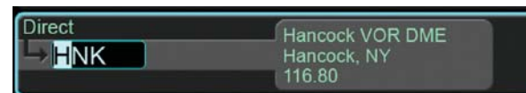
As an example, the logical GeoFill choice based upon the existing route is HNK rather than an irrelevant waypoint such as HM – Haneida NDB in Japan which an older system would have suggested because it is alphabetically ahead in the database.
