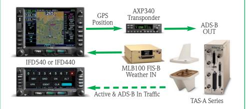
Avidyne provides a full suite of ADS-B IN and ADS-B OUT capable units that comply with impending mandates and provide traffic & weather information on Avidyne displays.
