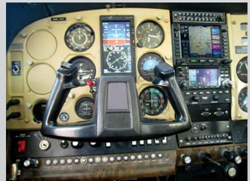
With the addition of an interface to the Aspen EFD1000 Pro, the DFC90 is becoming available to a growing list of aircraft including the Cessna 182 (above), the Beech Bonanza, and the Beech Baron.
