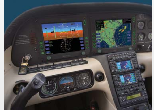
The DFC90 was initially certified as a replacement for the STEC55X in Entegra-equipped Cirrus SR20 & SR22 aircraft.
