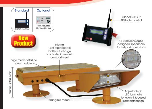
Avlite's solar powered, wireless controlled LED floodlight has been specifically designed for helipads to provide uniform surface lighting where the TLOF and FATO lights need to be supplemented with floodlighting. It offers a solar-powered, LED based solution to the ICAO touchdown and lift-off area perimeter floodlights.
