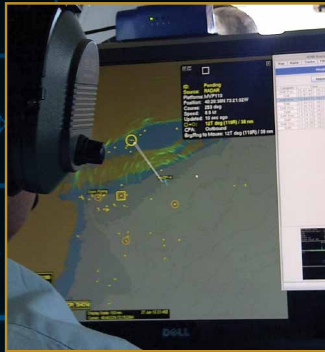
RDR-1700B(V)1 SHARC display during ISAR collection
