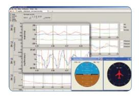
GYRO-VIEW 2.5 provides an easy to use graphical interface to display, record and analyze all of the VG800 measurement parameters.
