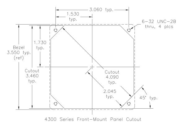
**Figure 2.3: Front Mount Panel Cutout Dimensions**
