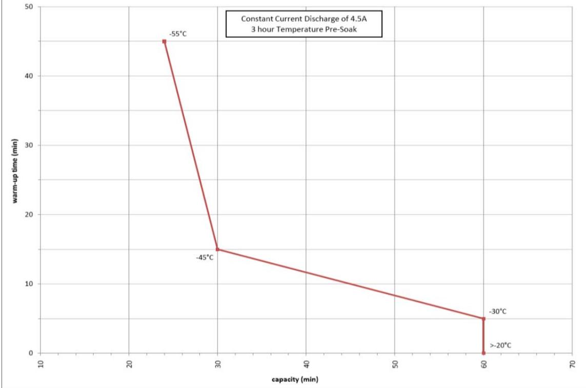
**Figure 4.3 Nominal Battery Capacity versus Warm-up Time**
