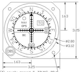
(3) equally spaced 6-32UNC $-2B^{-1}$  threaded holes on 3.500 dia. B.C.
