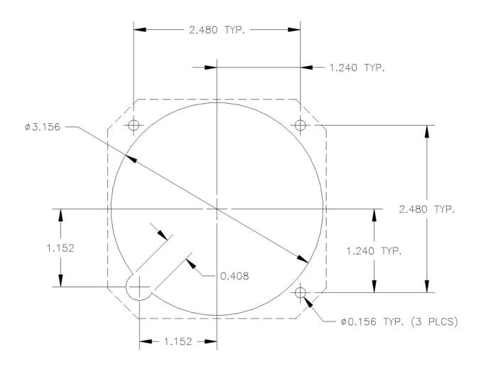
FIGURE 3-2: CUTOUT DIMENSIONS FOR PANEL MOUNTING
