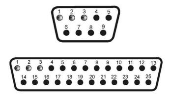
FIGURE 3-1: REAR VIEW OF MATING CONNECTORS
