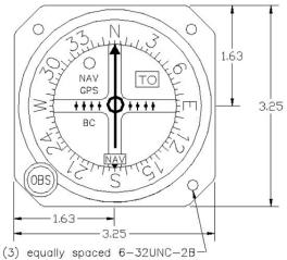
(3) equally spaced 6-32UNC-2Bthreaded holes on 3.500 dia. B.C.
