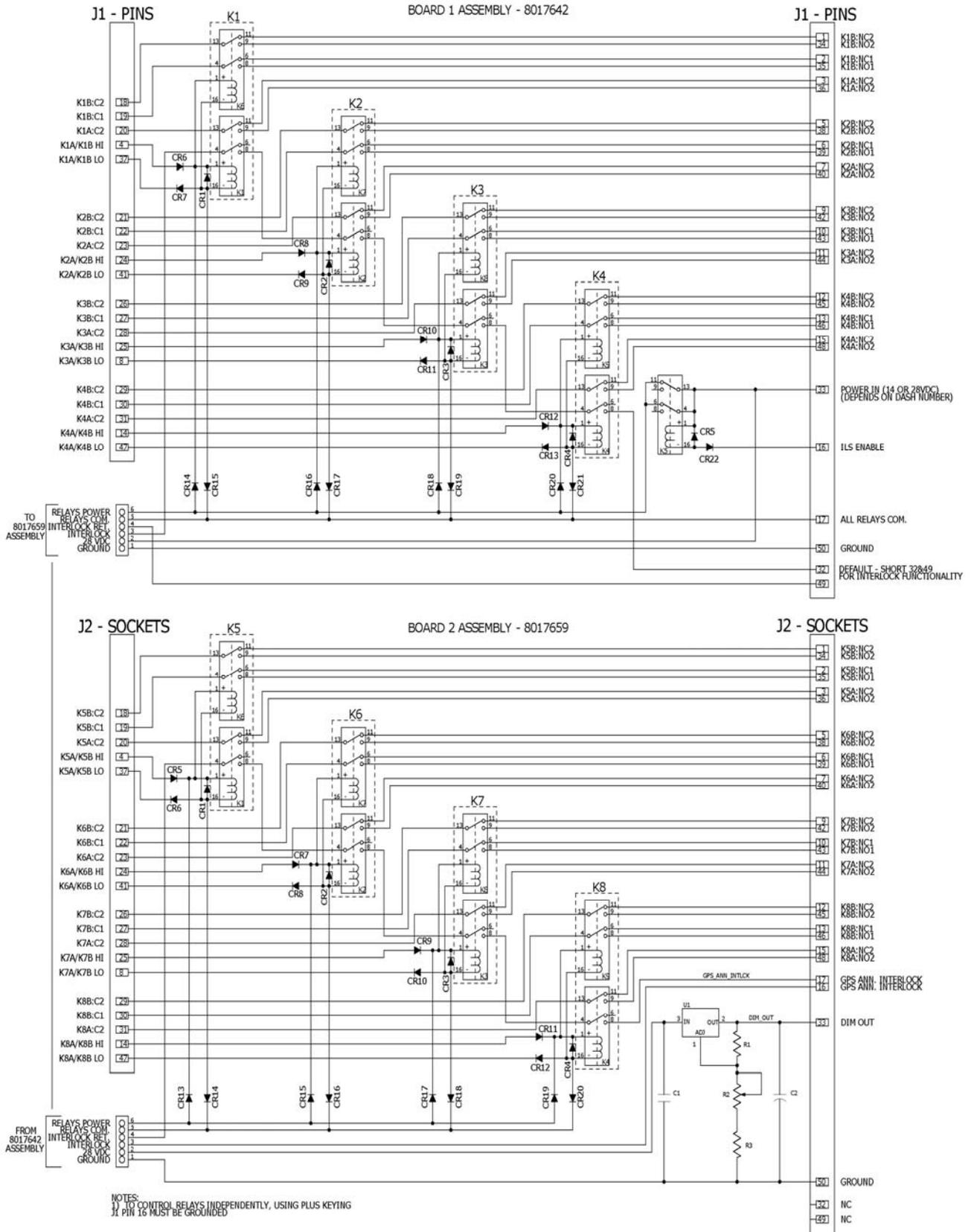
**FIGURE 3.3 SCHEMATIC DIAGRAM, MD41-24P() 24 POLE RELAY UNIT**
