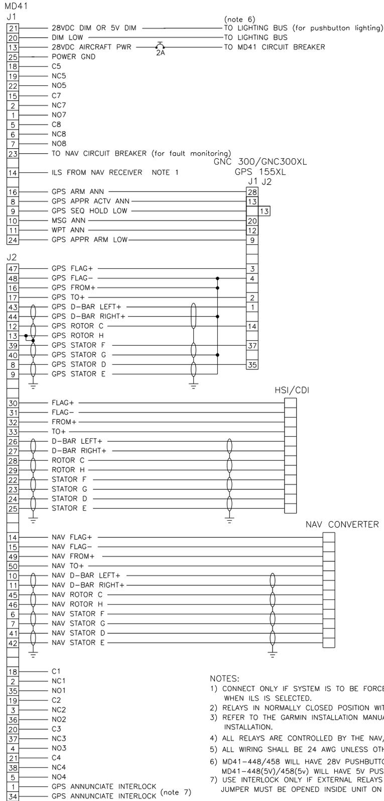
**FIGURE 3-6 WIRING DIAGRAM, MD41-448/458, GARMIN GPS 155XL, GNC 300 / GNC 300XL (28V)**
