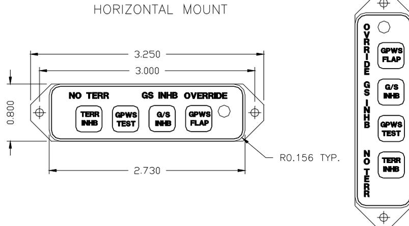
Note 1: Use two 4-40 X 3/8" Flat Head Phillips Screws for Mounting
