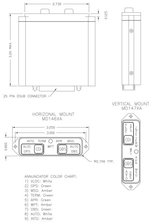
Note 1: Use two 4-40 X 3/8" Flat Head Phillips Screws for Mounting
