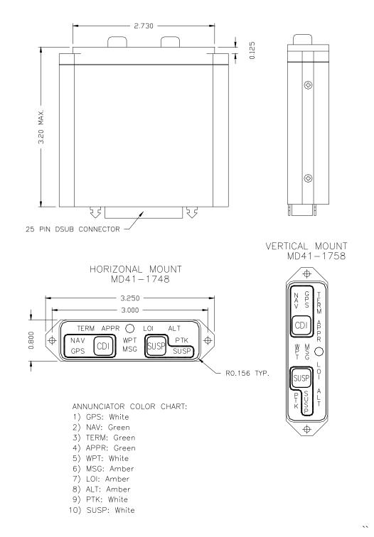
Note 1: Use two 4-40 X 3/8" Flat Head Phillips Screws for Mounting
