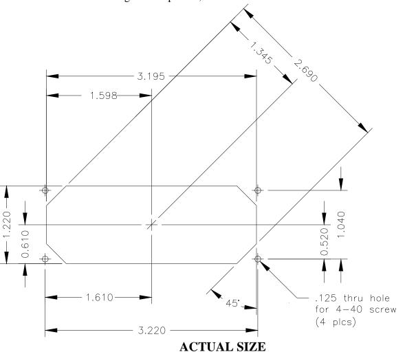
Note 1: Use four 4-40 X 3/8 to 1.0" Flat Head Phillips Screws for Mounting, MCI PN 7016165 (supplied). MD155 punch is available for hole cutout.
