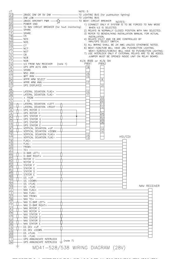
FIGURE 3-6 WIRING DIAGRAM, MD41-528/538/528(5V)/538(5V) KLN 89B or KLN 94 (28V)
