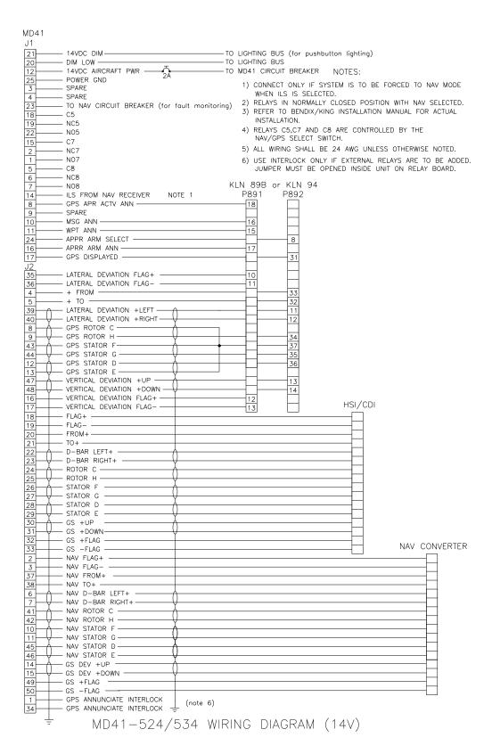
FIGURE 3-5 WIRING DIAGRAM, MD41-524/534 KLN 89B or KLN 94 (14V)
