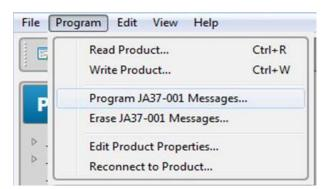
If a new audio file is selected, it may be played using the arrow to the right of the Message line, and uploaded to the JA37-001 using the 'Program' menu and selecting program JA37-001 Messages...'.
