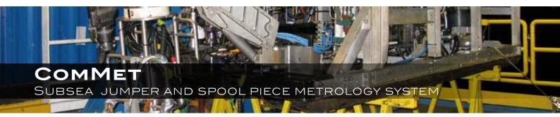
**ComMet** is designed to acquire accurate and traceable dimensional measurements of subsea structures, generally used in the design and production of interconnections between those structures.
