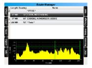
The AirScout LSA Moving Map is an affordable moving map system for light and sports aircraft (LSA). The AirScout LSA is a self-contained, rugged, panel mount system with a built-in high precision GPS receiver. The system integrates a variety of maps, with user selectable overlays such as ATC, approach maps, terrain, traffic (FLARM, ADS-B). The AirScout LSA increases your situational awareness, improves safety and quickly helps you convey position and target information.
