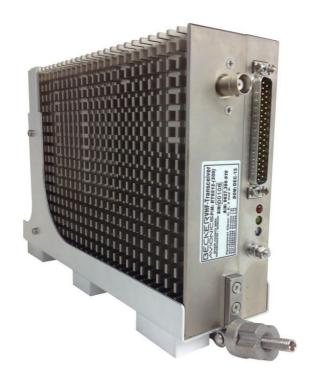
The remote-controlled VHF-AM transceiver is a half-duplex voice communication system in the standard avionics VHF frequency range 118.000...136.975 MHz (136.9916 MHz with 8.33 kHz channel spacing), or optional with extended frequency range up to 155.975 MHz and uses standard amplitude modulation (A3E). The VHF-AM transceiver is capable to operate in both, the 25 or 8.33 kHz channel spacing, is primarily intended for aeronautical operational control (AOC) and safety communications.
