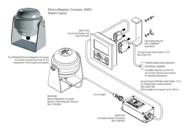
\*\*The MD71THD Control and Display Unit can display the heading in numeric form as a basic heading repeater (compass repeater). However, we always recommend using a dedicated Marine Data Heading Repeater suitable for the precise purpose to which it will be put (e.g. a repeater for steering the vessel; a repeater for taking bearings; a repeater to be mounted on the bridge wing, etc.)
